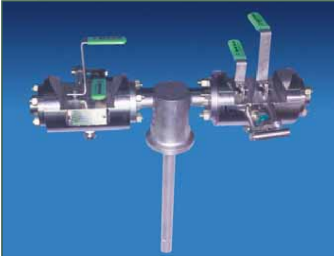
A TORBAR MACHINED FROM SOLID DUPLEX MATERIAL BAR WITH SPECIAL TECKLOK FLANGE RATED AT 455 BAR AND FITTED WITH DOUBLE BLOCK AND BLEED VALVES
