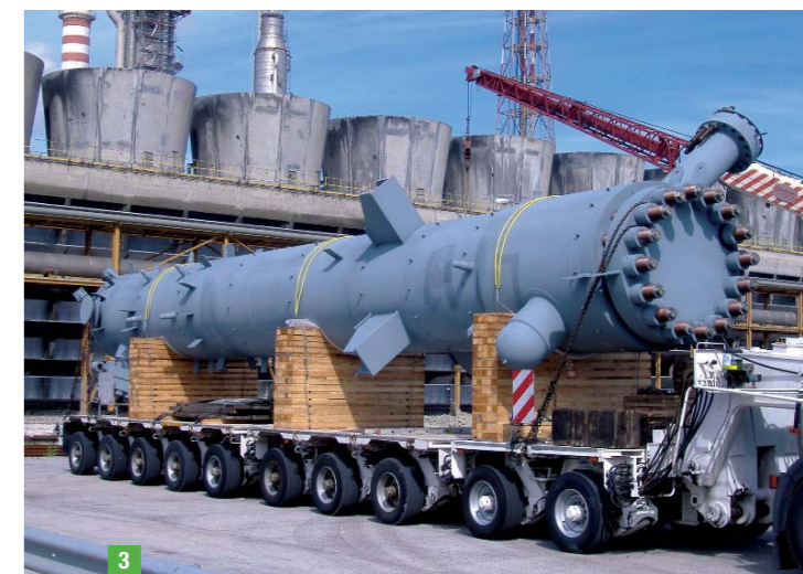
4 Secondary Reformer, SA 204 Gr. B, Technip - Wesfarmers CBSP, Australia
