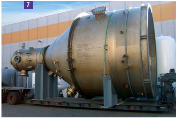
6 Solvent Dehydration Column and Crystallizer, Duplex 2205, Foster Wheeler - Indorama, Map Ta Phut Thailand 7 CTA Crystallizer, Foster Wheeler - Indorama, Map Ta Phut Thailand 8 Dehydration Column, Duplex 2205, AkerKvaerner - Petroquimica Suape, Brazil
