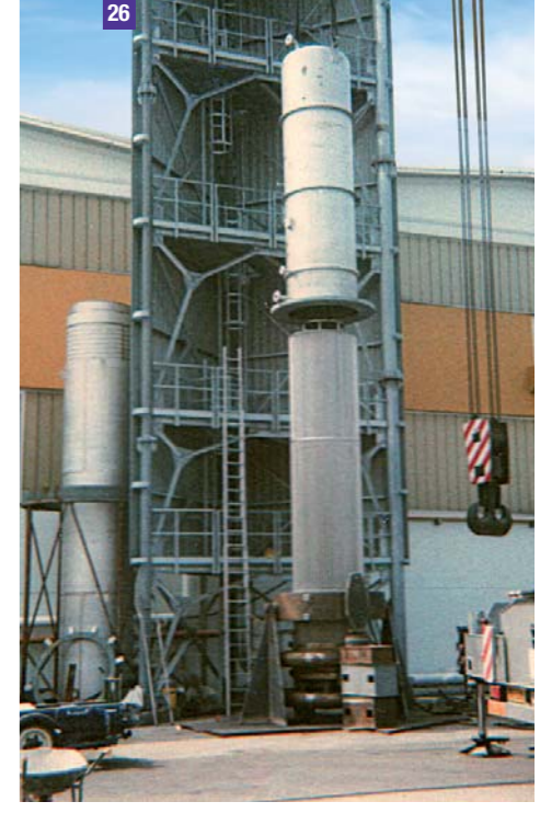
24 /25 /26 Reactor w/ Tube Bundle, 2.25 Cr alloy w/ C276 W.O., Agrolinz Melamin, Linz Austria
