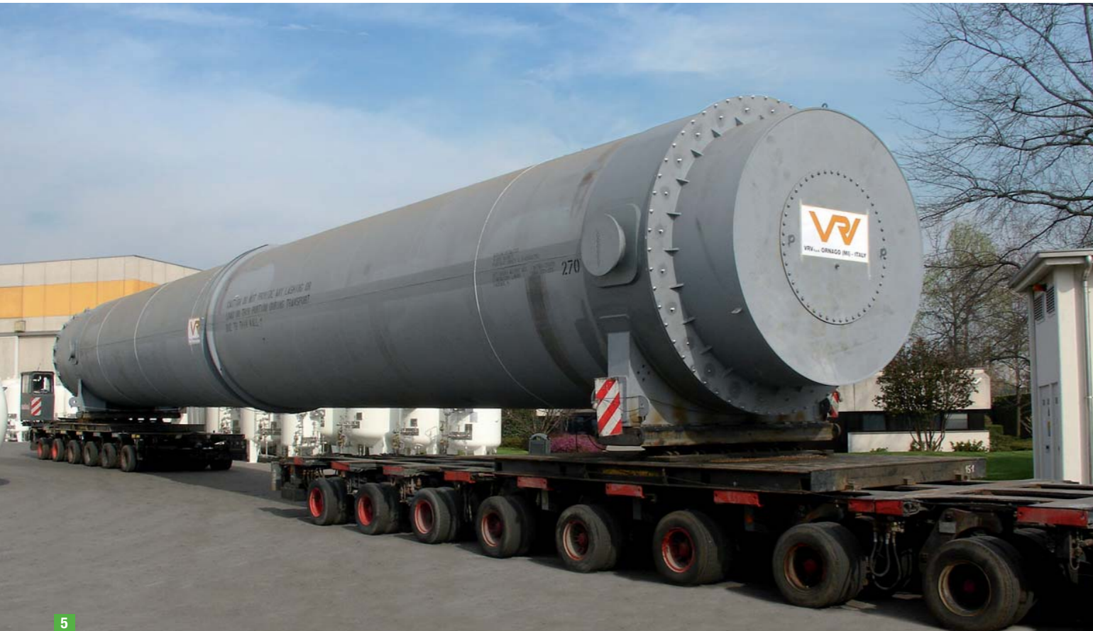
5 Ammonia Converter Basket (160 ton), 321 SS, Topsoe - Eagrum, Canada
