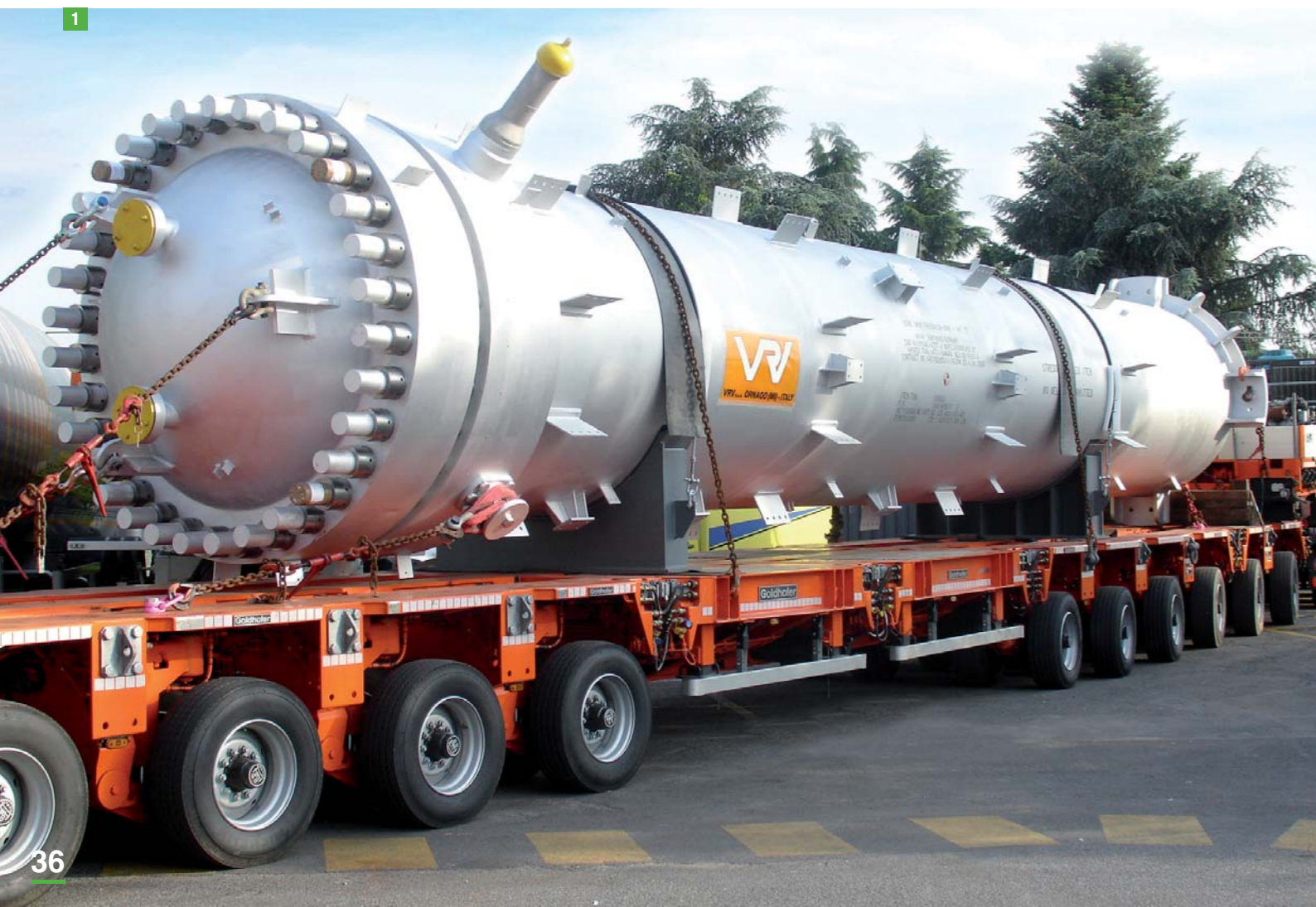
1 Ammonia Converter, 20MnMoNi 4 5, Uhde - Kuibyshev Azot, Kuibishevsk Russia
