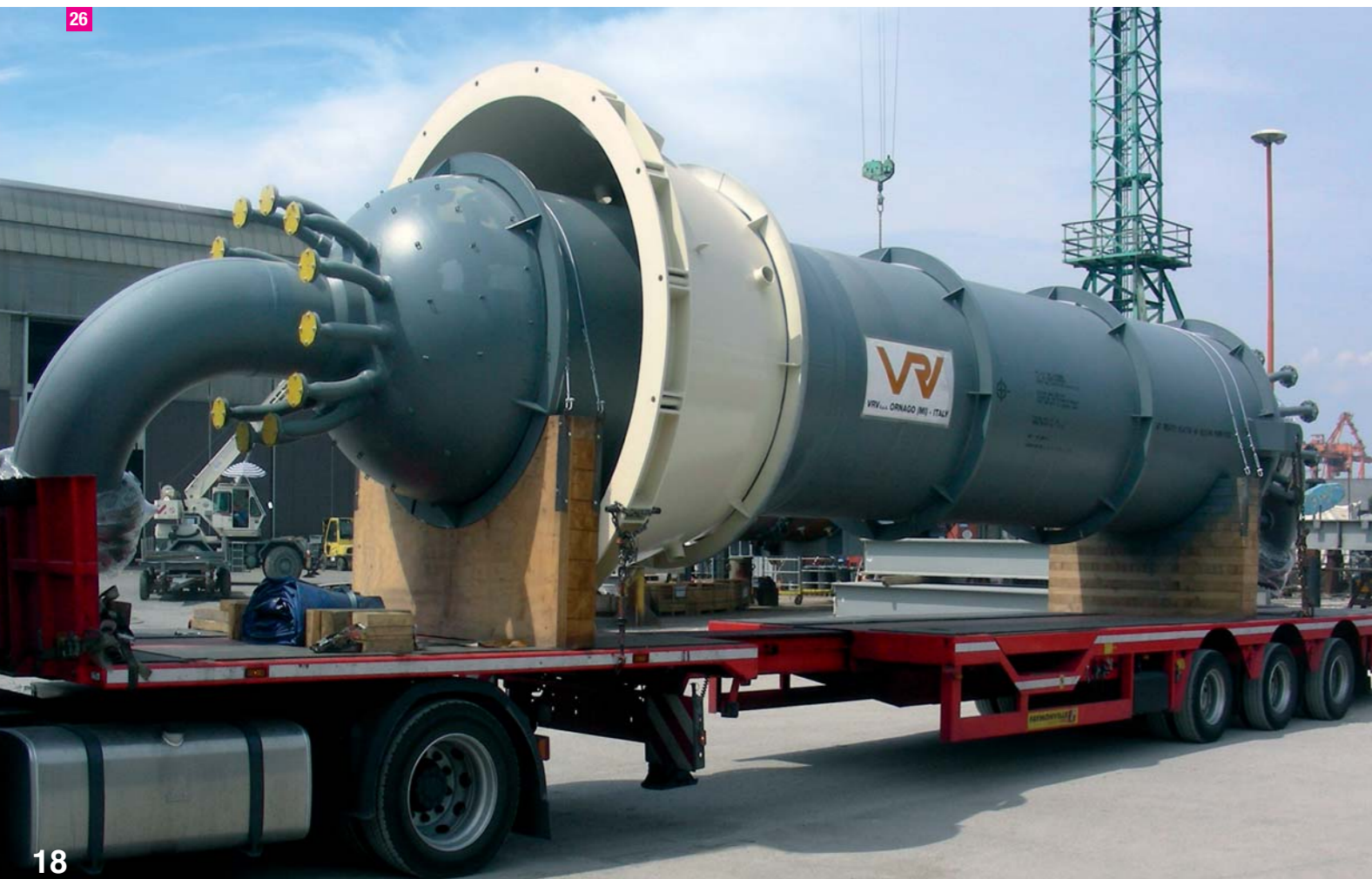
26 Octanizer Reactor, 2.25 Cr alloy, Sinopec - NIOEC, Shazand Arak refinery, Iran
