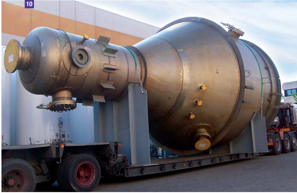
11 Dissolver Reactor (230 ton), 1.25 Cr alloy w/ 347 SS W.O., AkerKvaerner - Petroquimica Suape, Brazil
