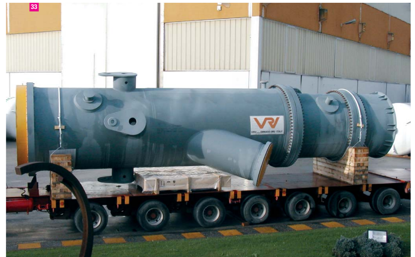
32 Orifice Chamber, CS w/ refractory lining, JGC Co. - ARAMCO, Rabigh refinery, Saudi Arabia
