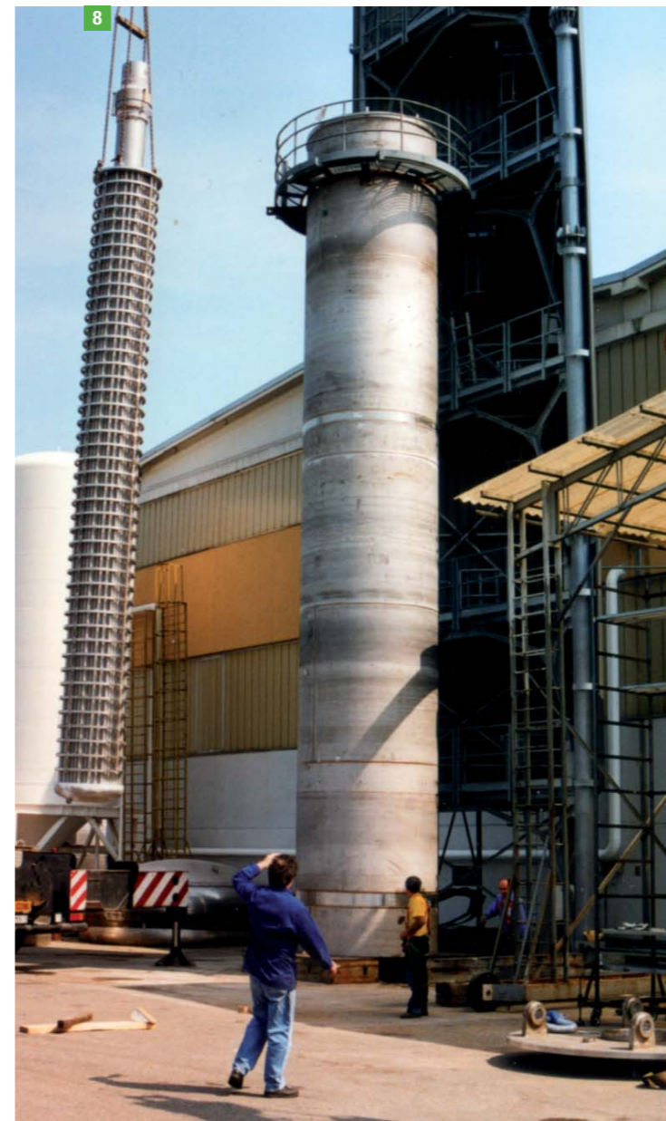
7 Ammonia Converter Basket, 304 SS, Uhde - Kuibyshev Azot, Kuibishevsk Russia
