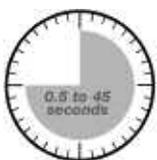
Turbulence and splashing can cause some fixed time response switches to produce false level alarms. Model 960 switches overcome this difficulty with an adjustable time delay feature.
