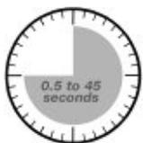
Turbulence and splashing can cause some fixed time response switches to produce false level alarms. Model 960/961 switches overcome this difficulty with an adjustable time delay feature.
